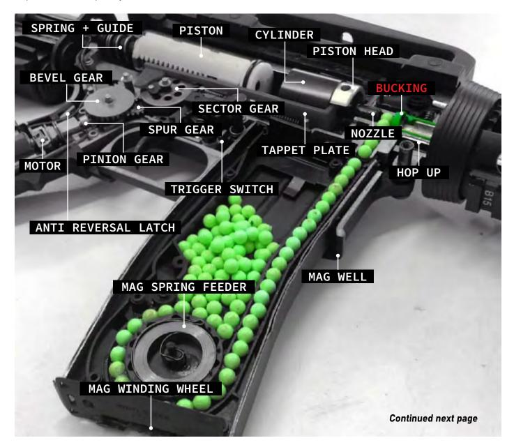
Softer buckings tend to grip the BB better, providing more backspin relative to the pressure applied. Finally, softer buckings tend to do better in colder weather, remaining more pliant and grippy where harder buckings become a little more brittle.
