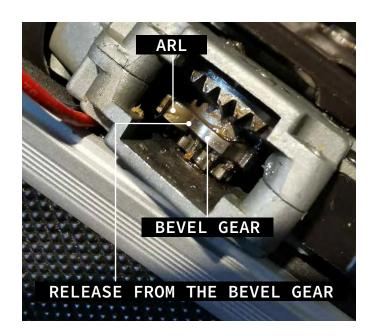
Solution is to trip the ARL (Anti Reversal Latch) allowing the gears to spin backwards until the piston is fully forward and the spring is no longer compressed.
